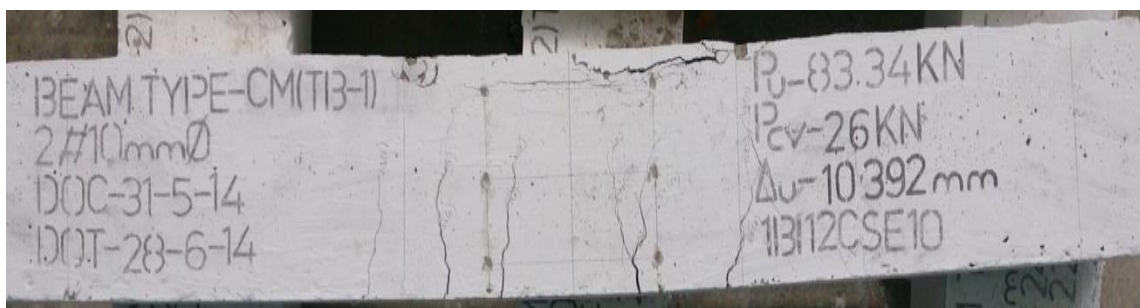
Fig 7: Crack Pattern Of Test Beams
